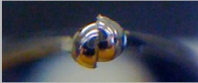
These tines are clearly misaligned when magnified. Without magnification, this is not easy to see. 95% of "smoothness" problems are exactly what you see above. The tines do not usually need smoothed, just realigned.
